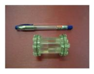
**Fig. 2.** The image quality phantom recommended by NEMA NU-4 2008.
